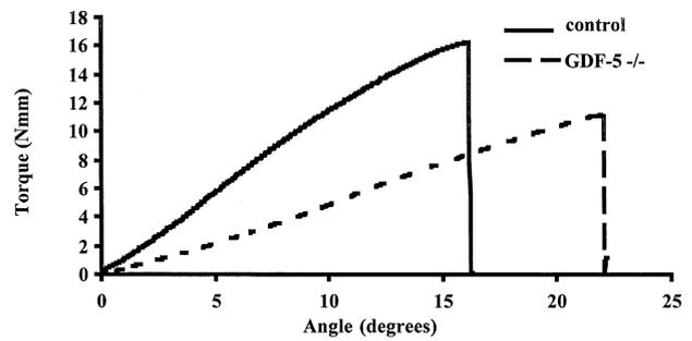
**Figure 2.** Representative torque vs. angle mechanical testing curves for control (solid line) and GDF-5-deficient (dashed line) femora.
